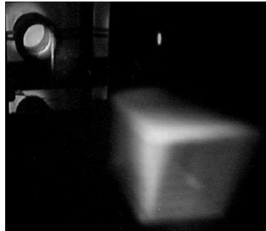
Fig.7. Pyramidal Cone Shape Image Formed by the Volumetric Rotating Scree
